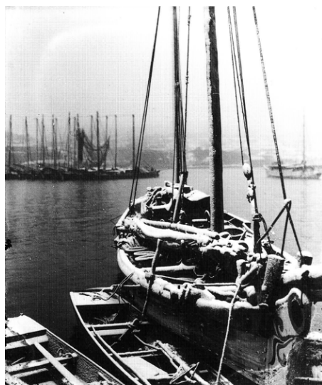
Figure 1. Utase boat in the harbour of Toba, early thirties. The particular shape of the bow is in the 'Aichi style' (Okada 1998, 37).
