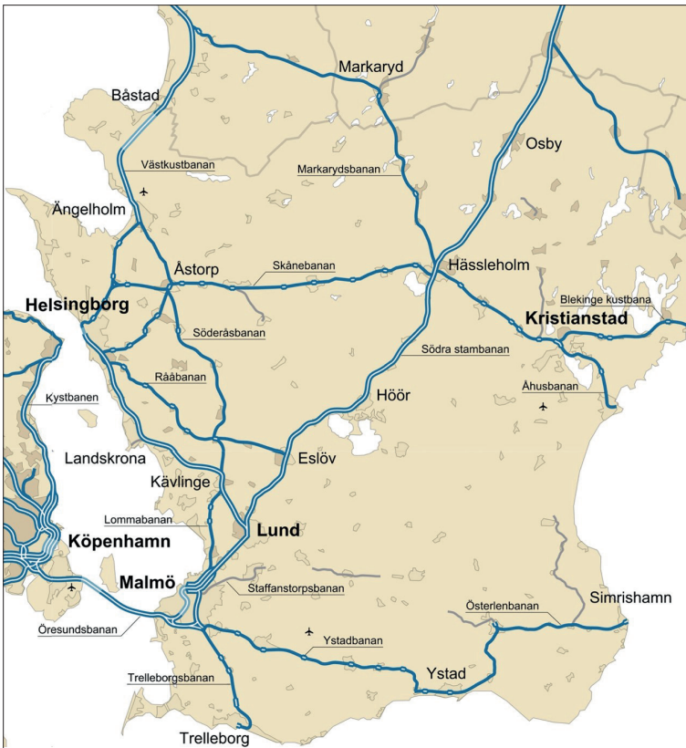
Figure 1 Railway network in Skåne and eastern Sjaelland (Denmark) showing single and double track (----- single track ===== double track)
