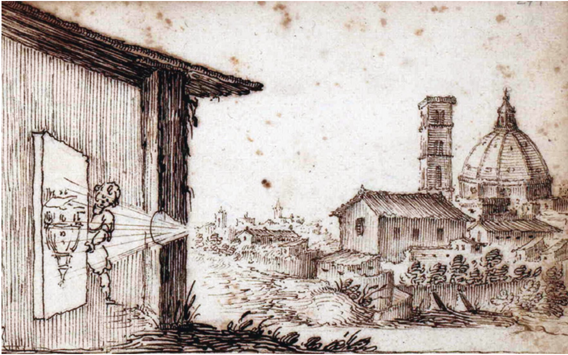
Figure 8 G. Parigi (ca 1600), Taccuino di arte militare , ms. Washington, Library of Congress, Rosenwald Collection, c. 249r: the camera obscura
