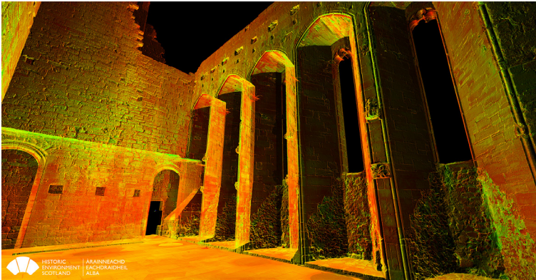
Figure 3 3D point cloud of the Palace Chapel at Linlithgow, Historic Environment Scotland
