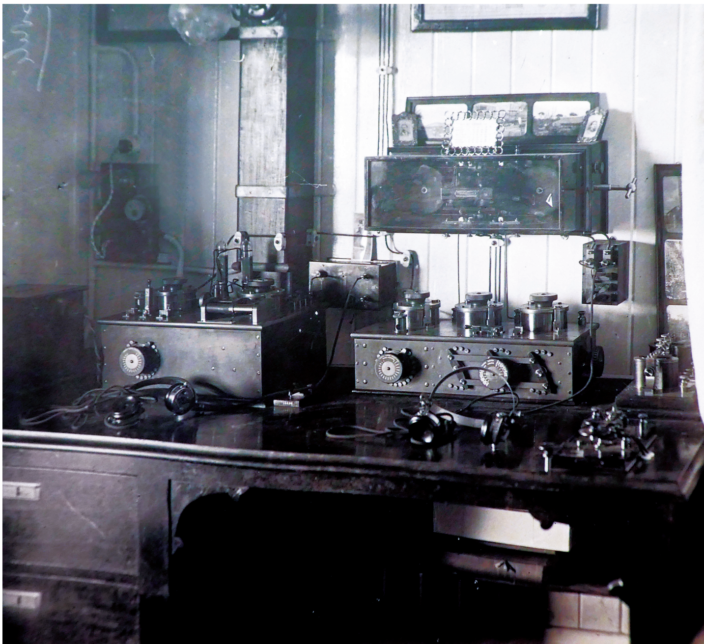
The detector is mounted on the wall; the tuner is sitting on the table underneath
