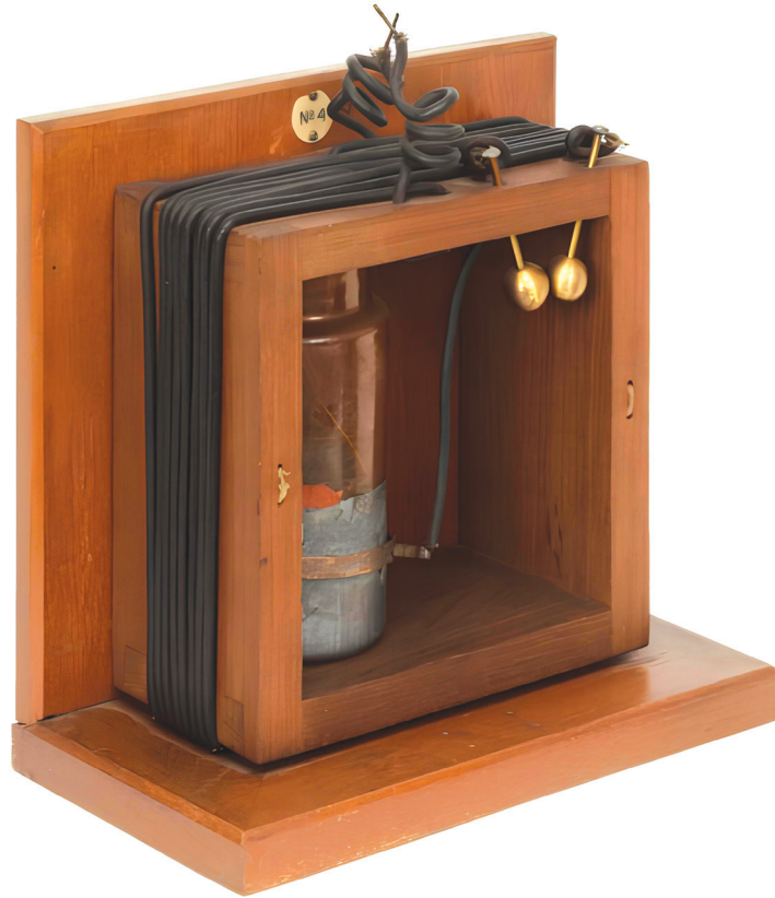
A reproduction of an experimental tuned transmitter circuit as described in patent no. 7777, issued to Guglielmo Marconi and the Marconi's Wireless Telegraph Company Ltd., 1932, inv. IGB 002137
