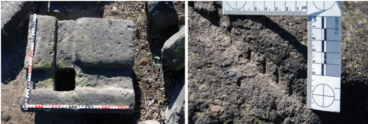
Figure 23 On the left side, the tuff ashlar A.5; on the right side, a detailed photo of the tool marks
