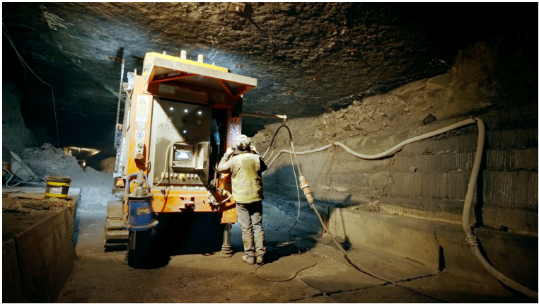
Figure 10 The automated saw used to cut the blocks of black marble
