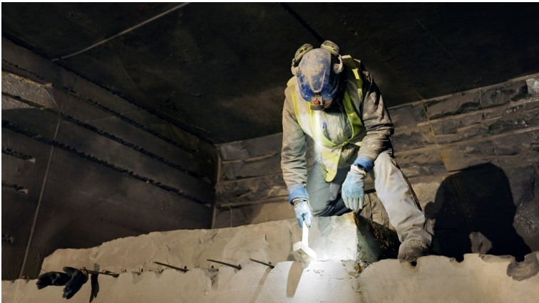
Figure 12 Use of wedges to detach a block of black marble
