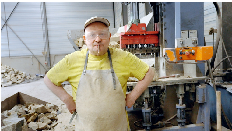
Figure 23 An operator of the cleaving machine that cuts rubble stone to size
