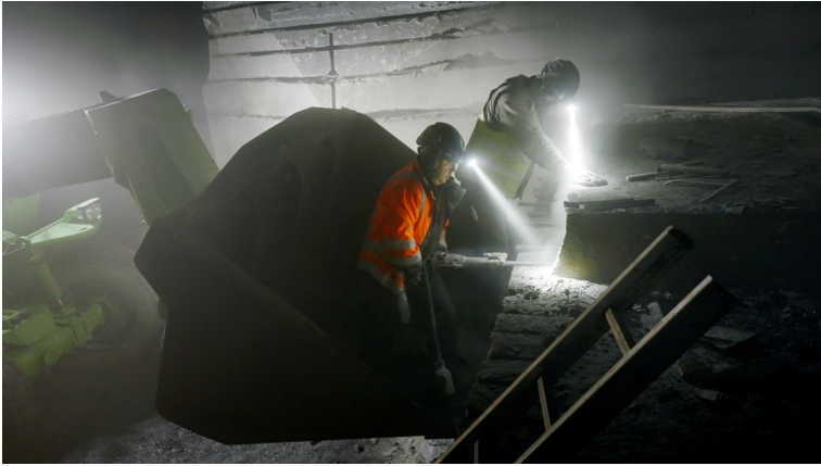
Figure 13 Drilling holes to detach a block of black marble
