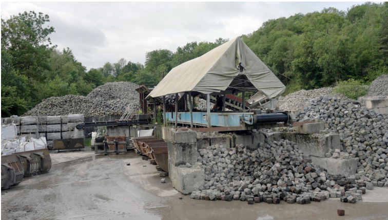
Figure 25 Conveyor belt used to sort salvaged paving elements according to type and dimensions
