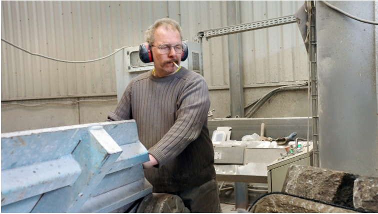
Figure 24 An operator of the cutting machine that is used to process reclaimed stone blocks
